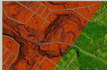
LiDAR is a remote-sensing technology that produces surface models from measured laser pulses emitted from a
