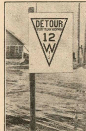
Detour Marker Placed along detour. To be followed in same way as Trunk Highway Marker.
