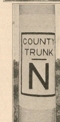
County Trunk Highway Marker Many counties are patrol maintaining their main highways and will mark these roads as above. The letter below is the county index to that special road and changes for each road.
